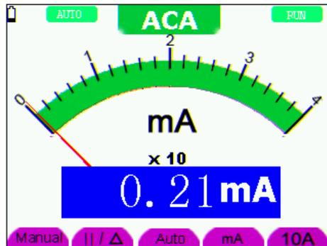
Figure 29: AC Current Measurement for <400 mA
