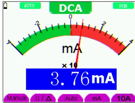
Figure 27: DC Current Measurement for <400 mA
