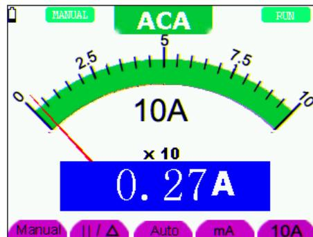
Figure 30: AC Current Measurement for <10 A
