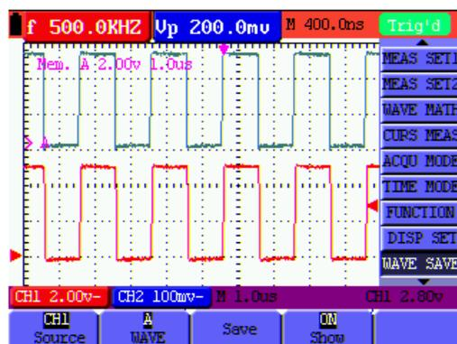
Figure 47: Waveform Saving
