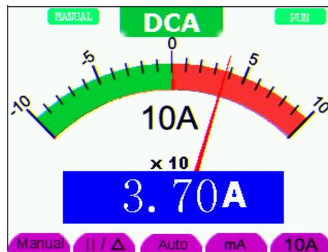
Figure 28: DC Current Measurement for <10A
