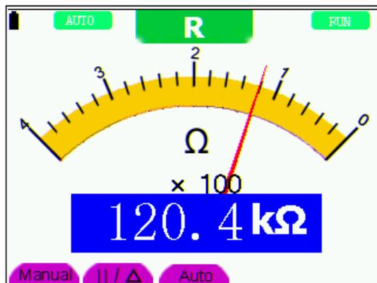
Figure 21: Resistance Measurement
