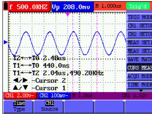
Figure 50: Use the Cursor for a Time Measurement
