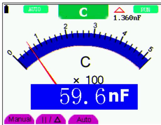
Figure 32: Relative Measurement
