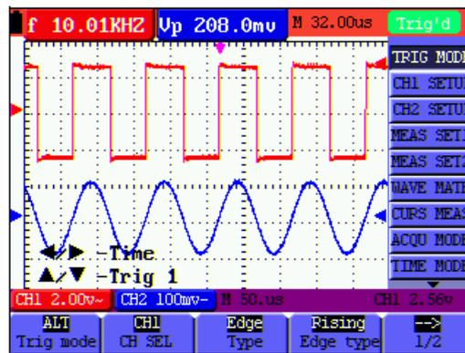
Figure 43: Alternate Trigger
