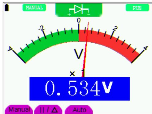
Figure 22: Diode Measurement
